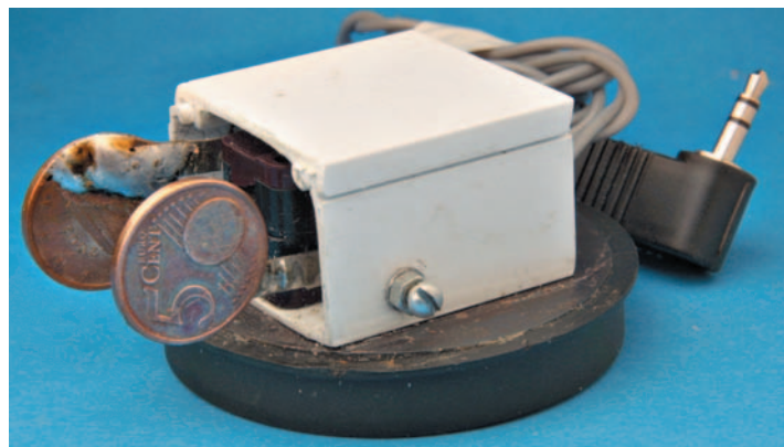
● With Tony EI5EM's 'Ten Cent' Euro-paddle idea you can make a small iambic c.w. keyer very cheaply with those spare coins lying around!
